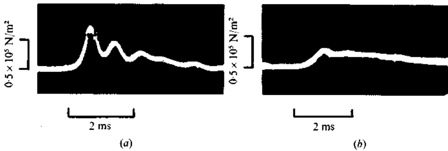
FIGURE 13. Evolution of the multi-soliton perturbation in a liquid with He bubbles. \sigma = 36 ; \sigma/Re = 0.14 ; \Delta P_0 = 1.74 \times 10^5 \text{ N/m}^2 ; l_0 = 0.15 \text{ m} .
